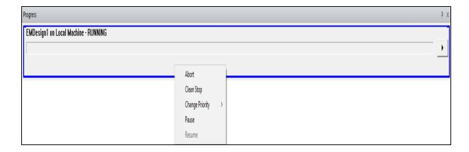
Right-click within the Progress window and select Change Priority > (Highest, Above Normal, Normal, Below Normal, or Lowest Priority), to change the priority of the associated solution. Altering the priority can be useful when multitasking, to free up resources from a computationally intensive application. Conversely, it can prevent less important programs from excessively slowing down the more intensive application.
