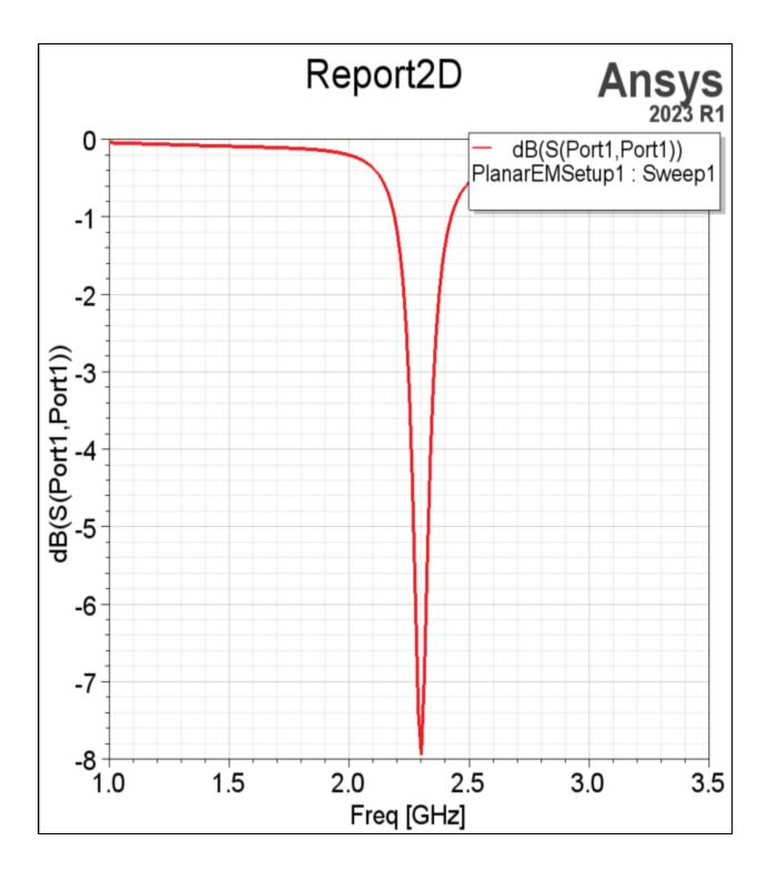
3. While the trace is selected, right-click anywhere within the **Report2D** window. Then select **Marker** > **Add Minimum**. An arrow will appear, indicating the lowest position from the line, along with a legend giving the marker's exact X,Y coordinates.
