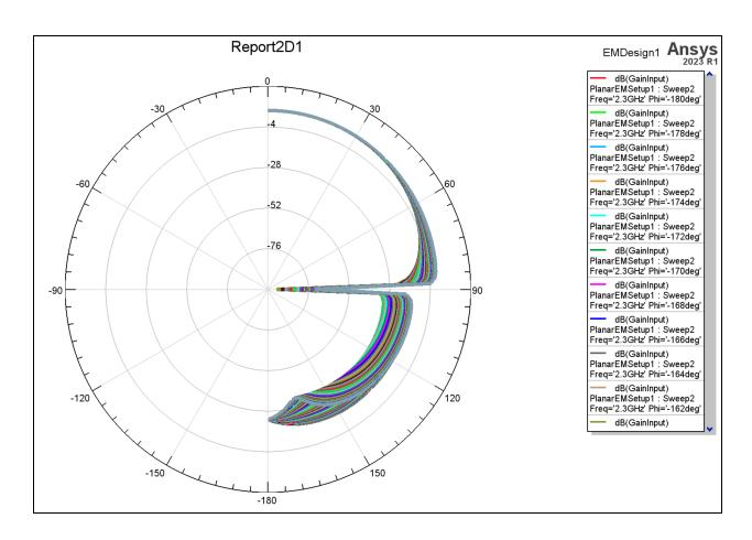
7. Double-click the Theta axis (i.e., the outer circumference of the plot) to open the **Properties** window.
