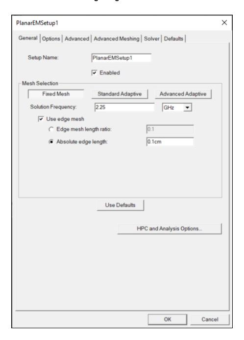
3. Click **OK** to close the **PlanarEM Setup** window and open the **Edit Frequency Sweep** window.
