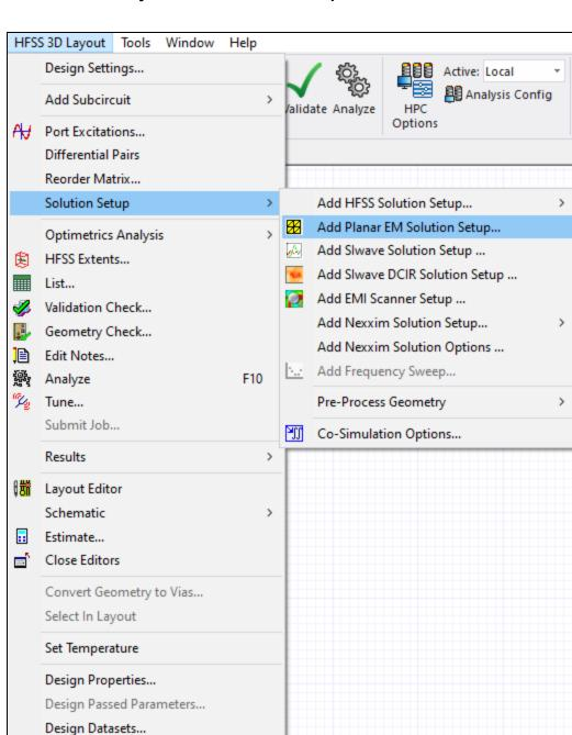
• From HFSS 3D Layout, select Solution Setup > Add Planar EM Solution Setup.
